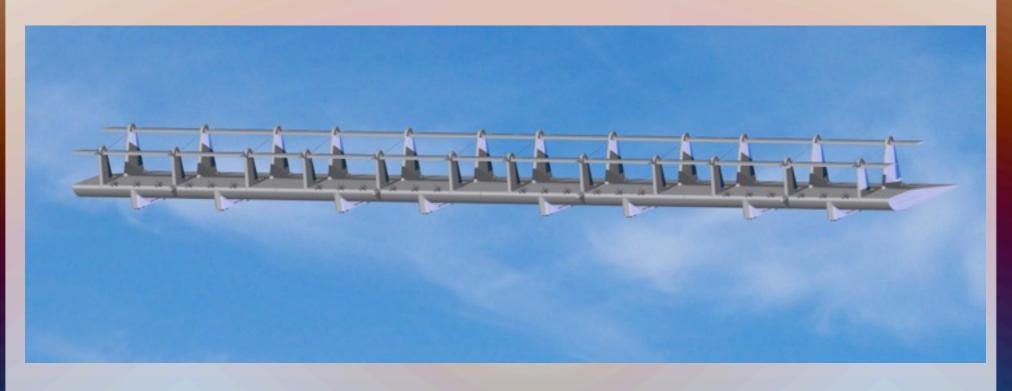
Folding wing extensions with additional tail plane, 260 ft span, 150 ft cord, 52 TEU or eight Abrams tanks.
